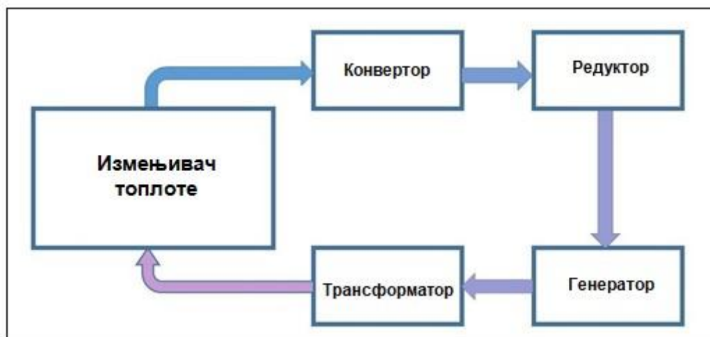
Figure no. 62: Cooling diagram of the main components in the gondola
