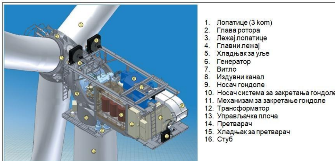
Figure no. 54: Wind turbine parts (WT)
